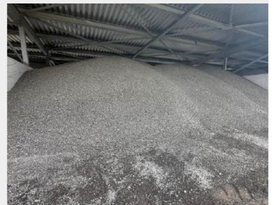
Trocken gelagertes RC-Kiesgemisch 0-16mm
